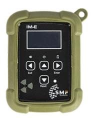
The IM-E personal electronic dosimeter is capable of measuring and recording the instantaneous dose rate and cumulative dose received by personnel in radiation environments. In hazardous situations, it can alert the user to potential threats through audible, visual, and vibration warnings. The radiation performance tests of the IM-E measurement device are carried out in ISO/IEC 17025 accredited laboratories in accordance with the IEC 61526 standard.
