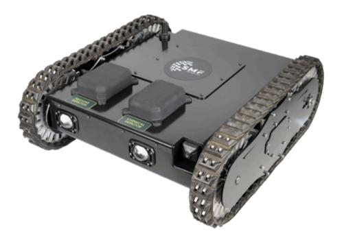
**RADROVER** provides a safe and effective means of performing radiological and nuclear measurement processes in challenging and hazardous areas, minimizing personnel risk. Thanks to its tracked system, it can operate optimally even under difficult field conditions. With a minimum of 90 minutes of continuous operation, it ensures sustainable use during missions.
