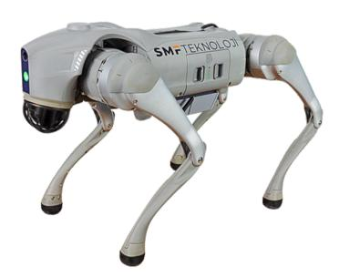
**RADROVER** provides a safe and effective means of performing radiological and nuclear measurement processes in challenging and hazardous areas while minimizing personnel risk. With a minimum of 60 minutes of continuous operation, a swappable battery design, and modular equipment integration, it offers flexible use for long-term and repetitive missions.
