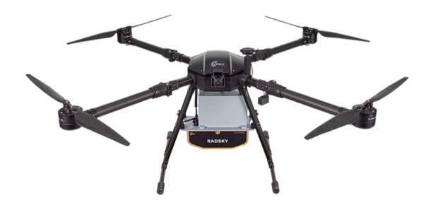
**RADSKY** provides a safe and effective means of performing radiological and nuclear measurement processes in challenging and hazardous areas. With a payload capacity of 10 kg, a flight time of up to 30 minutes, and a coverage area of 7 km<sup>2</sup>, it can carry out comprehensive scans along planned routes. Using backup battery system, it can be quickly redeployed to continue monitoring activities in additional areas.
